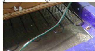
**Gambar 6. Kondensor Jenis Air Cooled Condensor**
